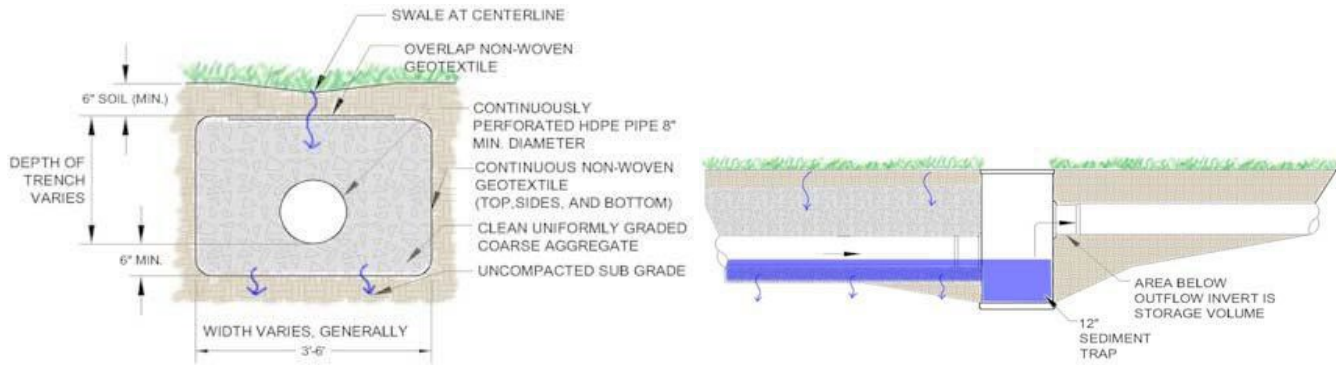
Figure 2: Infiltration Trench Diagram
